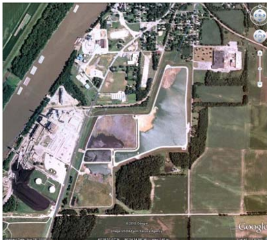
Aerial overview of Havana Power Station’s ash ponds. Note houses to the north (downgradient) from the East Ash Pond.
